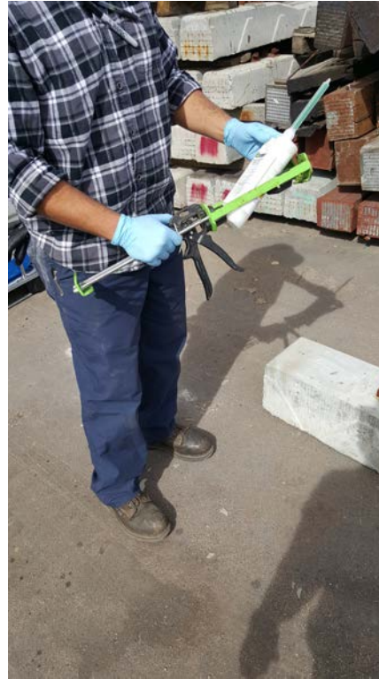
Place cartridge with mixer in manual applicator
