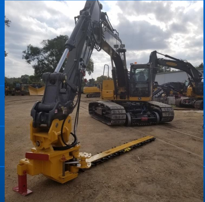
RCE - John Deere 210G Railavator with Undercutter Bar
