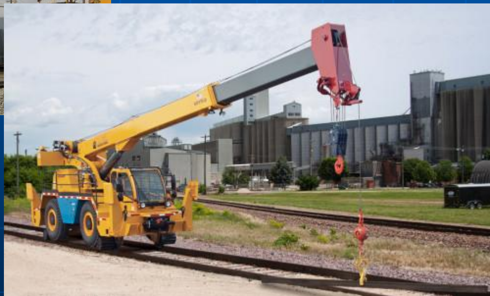
CD4430R 30T Rough Terrain Hi-Rail Crane
