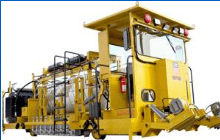
Series I CWR Rail Heater Car with Operator's Cab Upgrade
