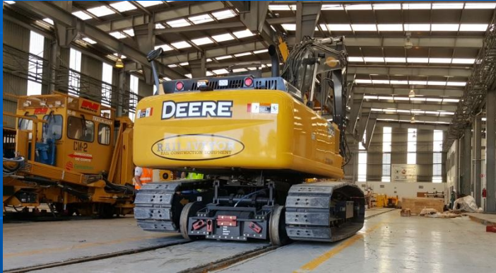
RCE - John Deere 210G Railavator with Hi Rail Equipment
